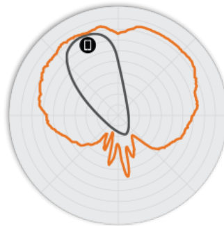
Figure 4. R510 2.4GHz Elevation Antenna Patterns
