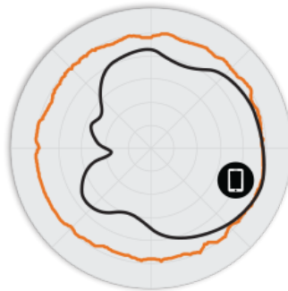
Figure 3. R510 5GHz Azimuth Antenna Patterns
