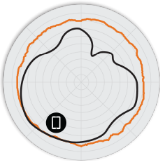
Figure 2. R510 2.4GHz Azimuth Antenna Patterns
