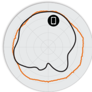
Figure 3. R320 5GHz Azimuth Antenna Patterns
