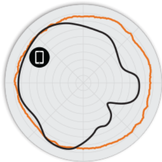
Figure 2. R320 2.4GHz Azimuth Antenna Patterns
