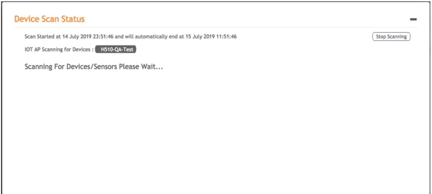
A device gets added to the Ruckus IoT Controller through Discover IoT Devices operations. If a device is pre-approved, the discovered device automatically joins the list of discovered devices. If the discovered device is not pre-approved, then you must select **Accept** or **Blacklist**. If the device is accepted, it joins the list of discovered devices.
