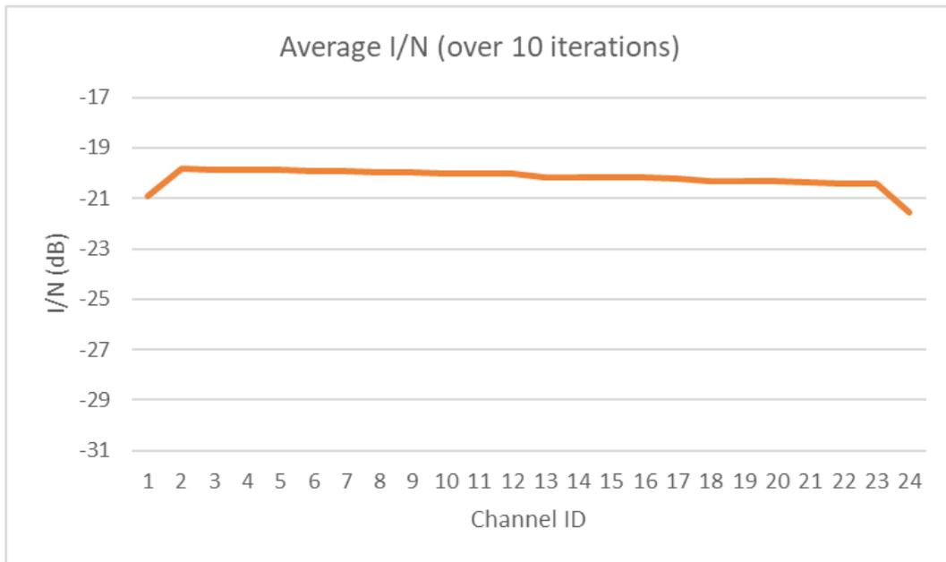
**Figure 58: IS-33e I/N per channel under mid active RLAN assumptions**
