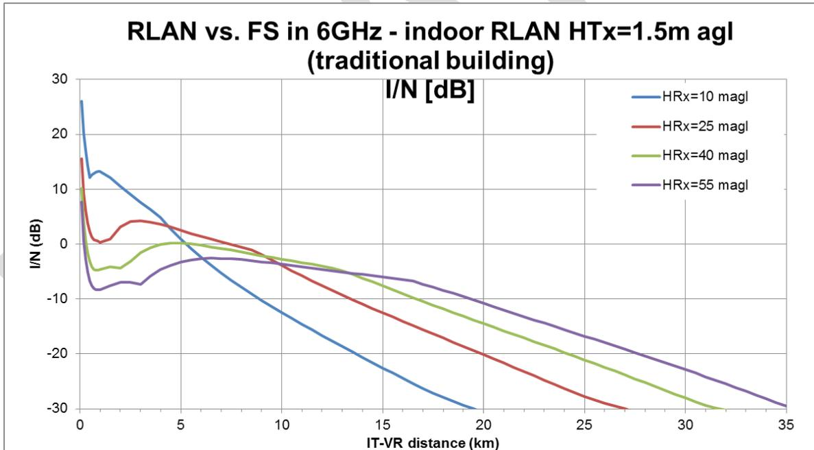
Figure 24: I/N at FS in dependence of RLAN distance in 0° azimuth direction of FS main beam (indoor RLAN @ 1.5 m, traditional building type)
