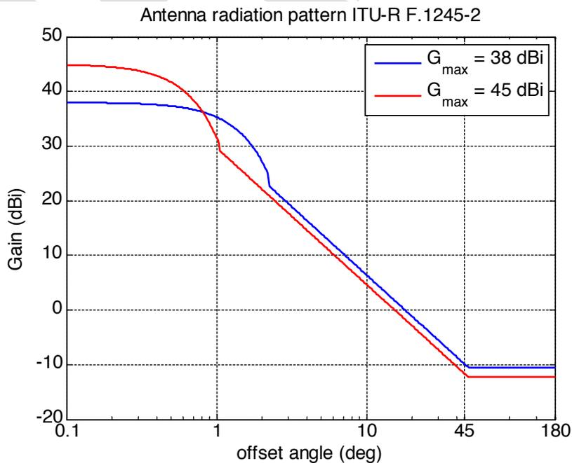
**Figure 6: Antenna radiation pattern of PP FS system for aggregate interference according to Recommendation ITU-R F.1245-2 at the band centre frequency of 6.175 GHz**
