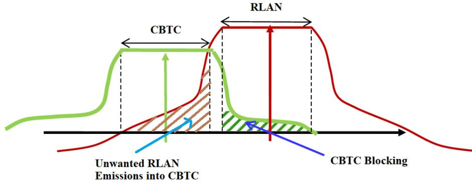
**Figure 79: Unwanted emission from RLAN into the CBTC channel as well as the CBTC blocking**
