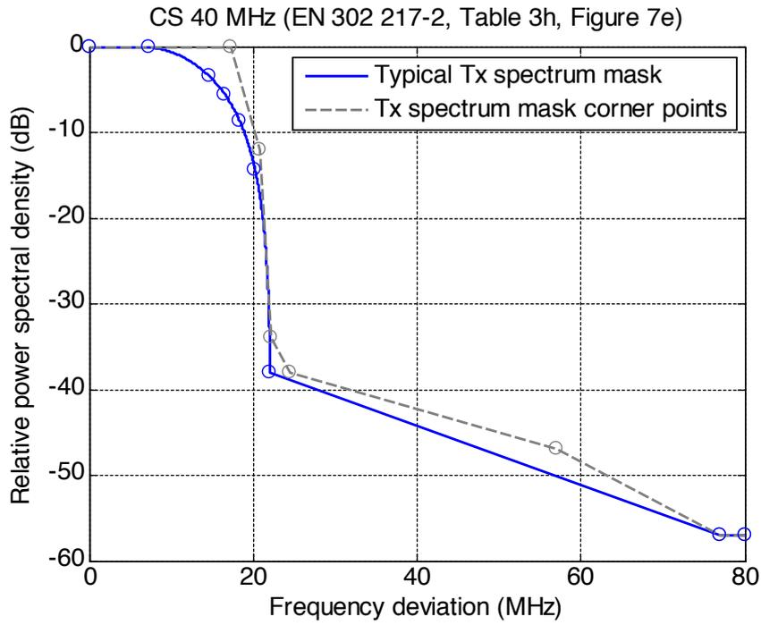
Figure 7: Typical transmitter spectrum mask for FS systems with channel spacing 40 MHz
