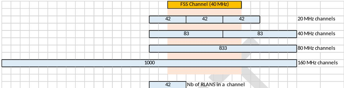
**Figure 107: RLAN channels incident to a 40 MHz FSS receiver bandwidth**
