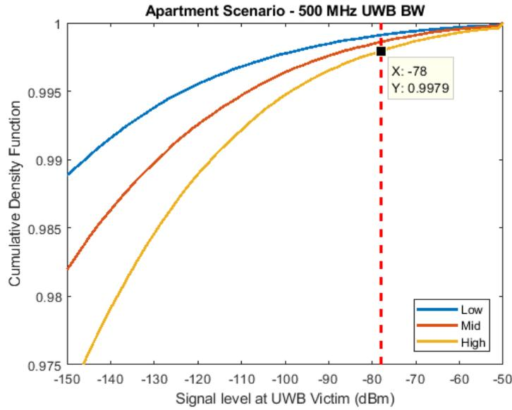
Figure 94: Monte Carlo results UWB apartment block scenario - 500 MHz UWB bandwidth
