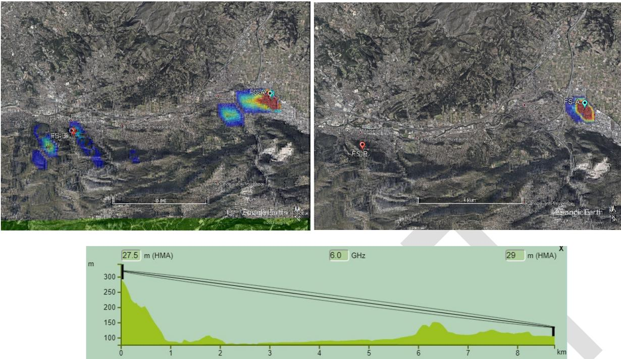
**Figure 52: Fixed link 3 at Marseille. Top left: Outdoor RLAN impact on the fixed link, Top right: Indoor RLAN impact on the fixed link. Bottom: Fresnel zone and path profile**
