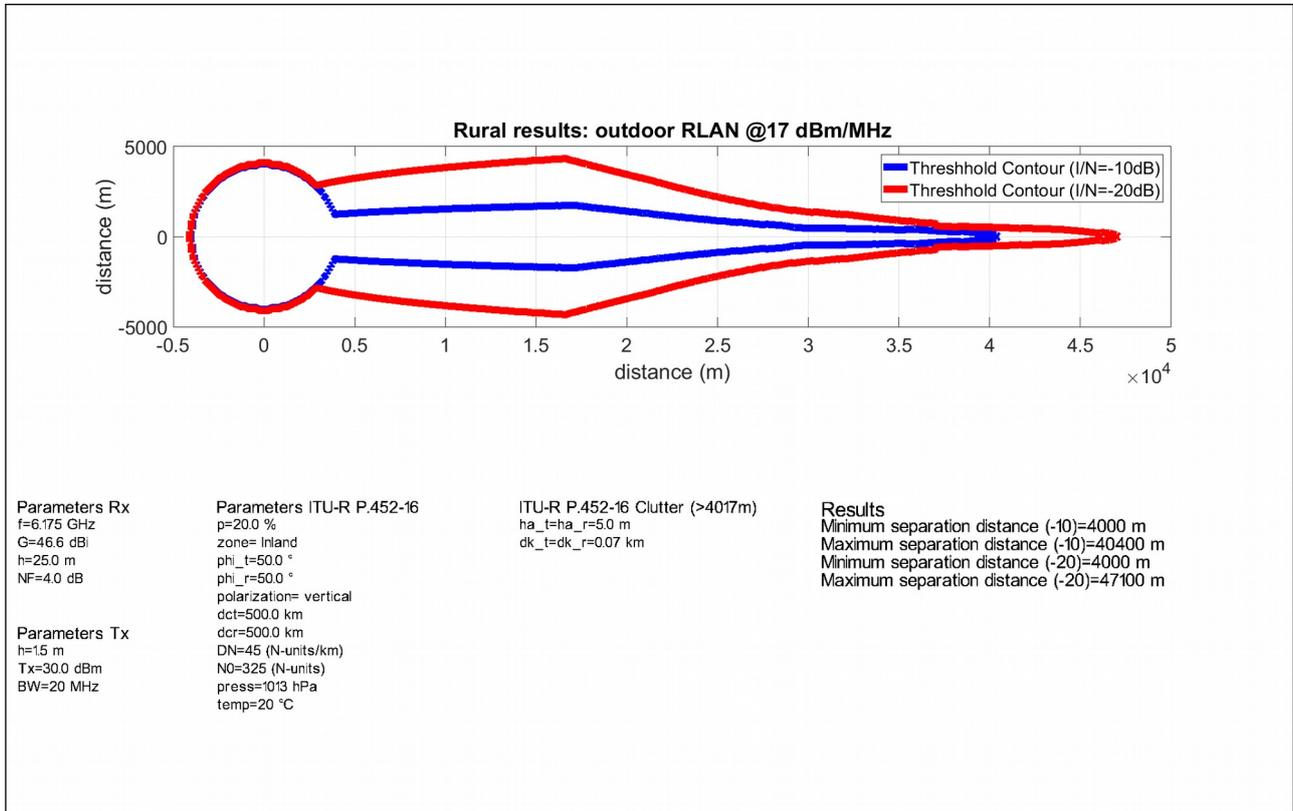
Figure 20: Rural results - outdoor RLAN @ 17 dBm/MHz e.i.r.p.
