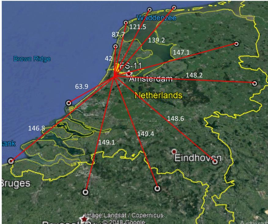
**Figure 32: Geographic location of RLANs that overlap frequencies with Netherlands FS 11 at the perimeter of 150 km radius (distance, in km, of each RLAN to the FS is indicated)**
