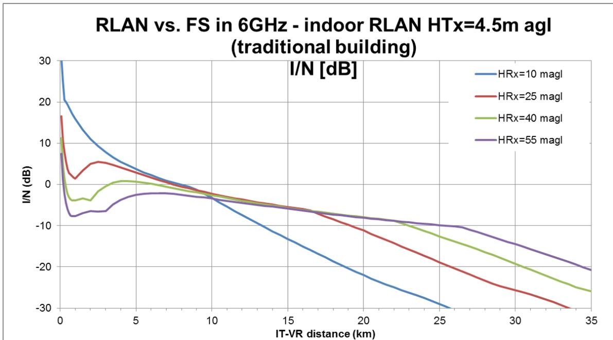
Figure 25: I/N at FS in dependence of RLAN distance in 0° azimuth direction of FS main beam (indoor RLAN @ 4.5 m, traditional building type)
