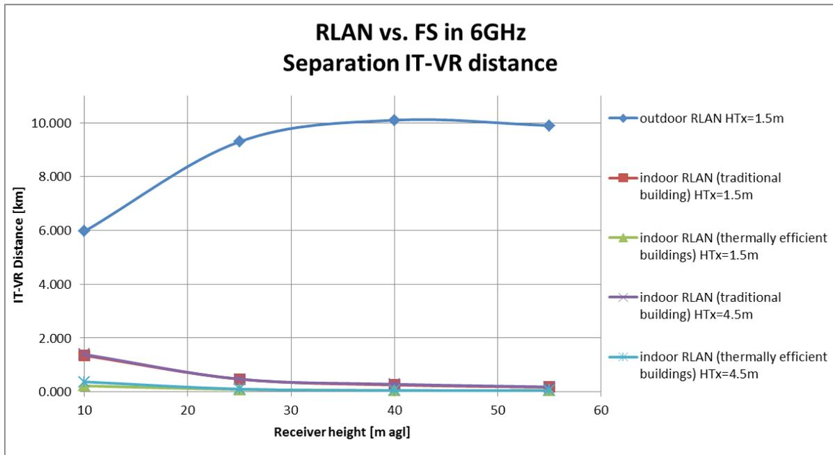
**Figure 31: Dependency of critical peak radii on the FS receiver height and RLAN environment for  $I/N = -10\text{dB}$  and minimum interference scenario**
