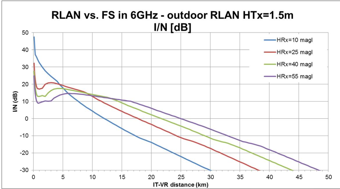
Figure 23: I/N at FS in dependence of RLAN distance in 0° azimuth direction of FS main beam (outdoor RLAN @ 1.5 m)
