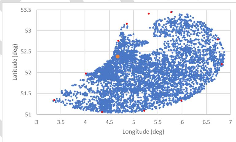
**Figure 33: Density of 6249 instantaneously transmitting RLANs with frequency overlap in 150 km radius of Netherlands FS 11 receiver**
