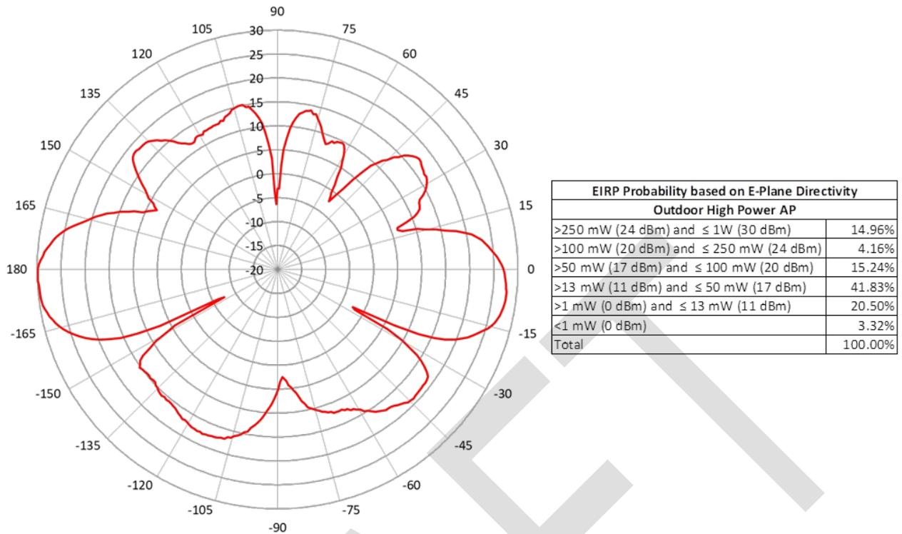
Figure 105: e.i.r.p. probability based on E-plane directivity for outdoor high power AP
