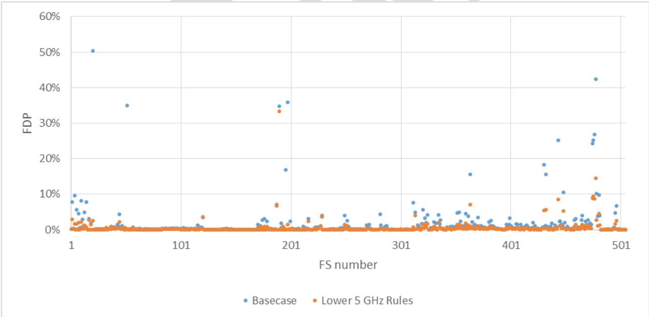
**Figure 47: FDP for each of the 505 FS receivers in the UK with lower 5 GHz rules**
