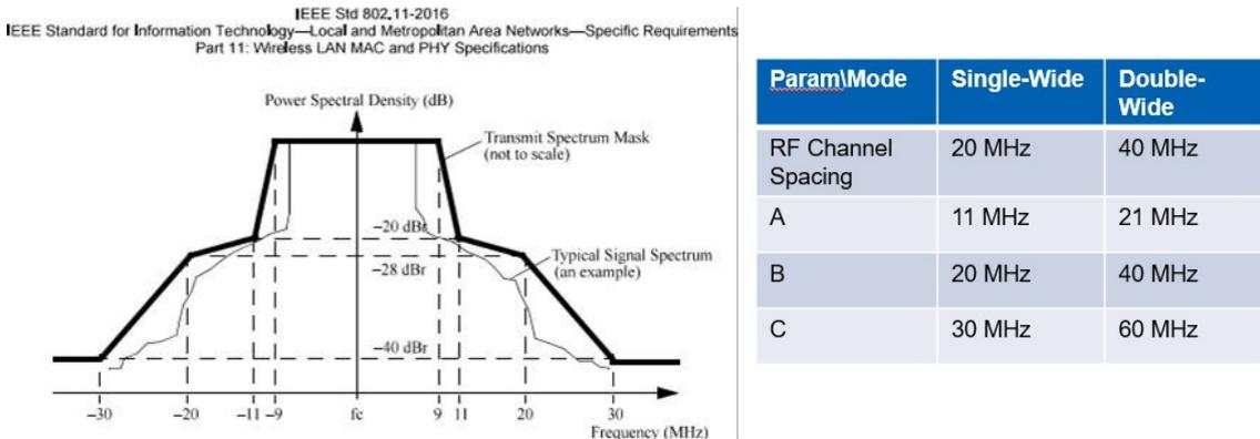
Figure 90: IEEE 802.11 Out-of-Band (OoB) emission requirement for OFDM transmissions
