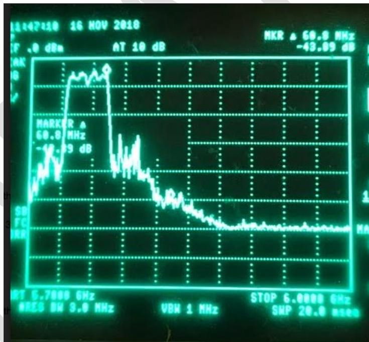
Figure 91: RLAN spectrum mask measurement
