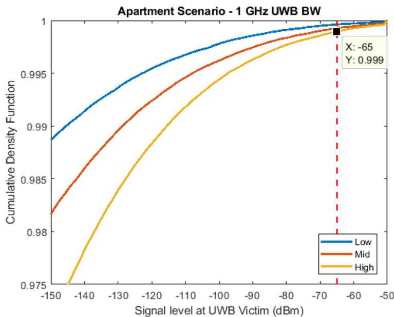
Figure 95: Monte Carlo results UWB apartment block scenario - 1 GHz UWB bandwidth
