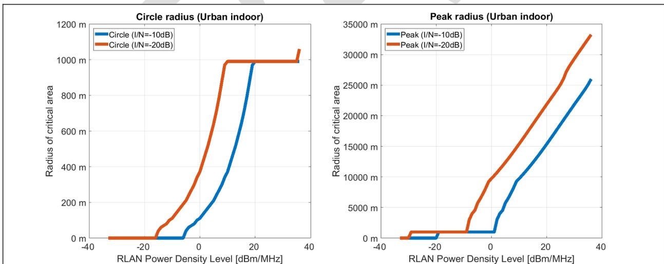
**Figure 28: Dependency of critical radii on the RLAN power density indoors**
