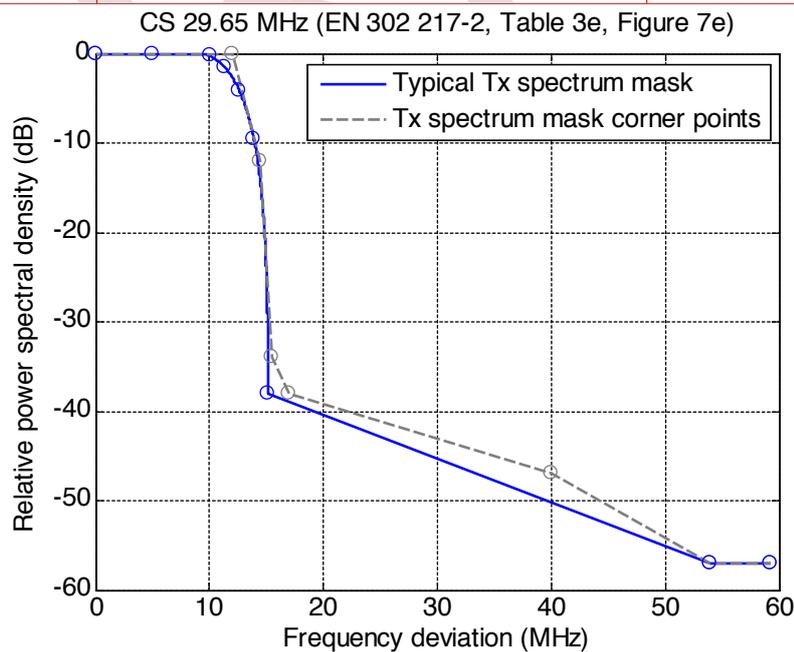
**Figure 9: Typical transmitter spectrum mask for FS systems with channel spacing 29.65 MHz**
