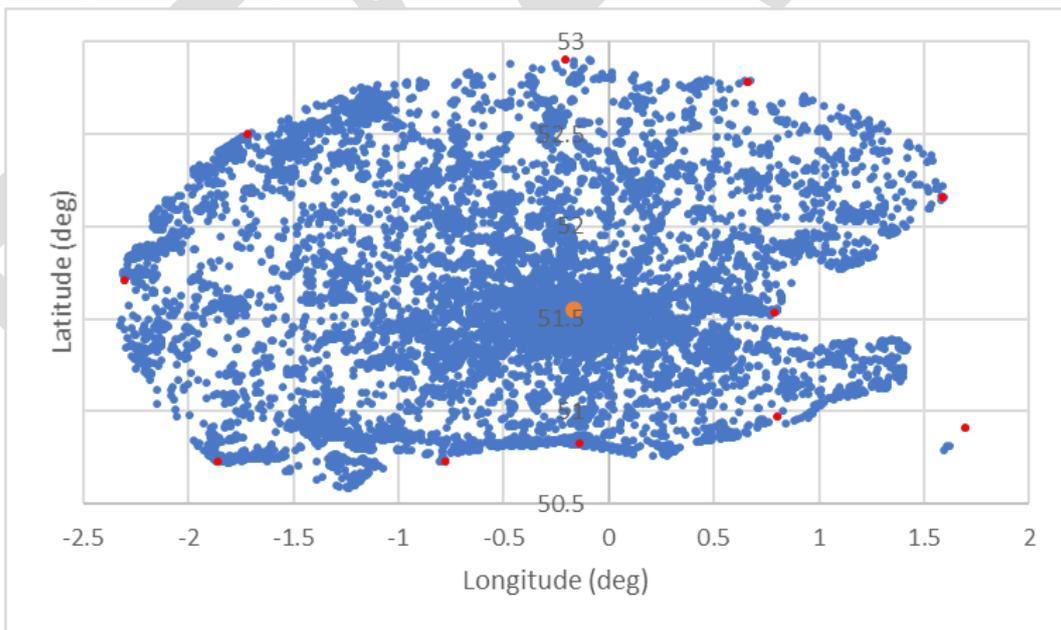
**Figure 40: Density of 17 066 instantaneously transmitting RLANs with frequency overlap in 150 km radius of UK FS 477 receiver**
