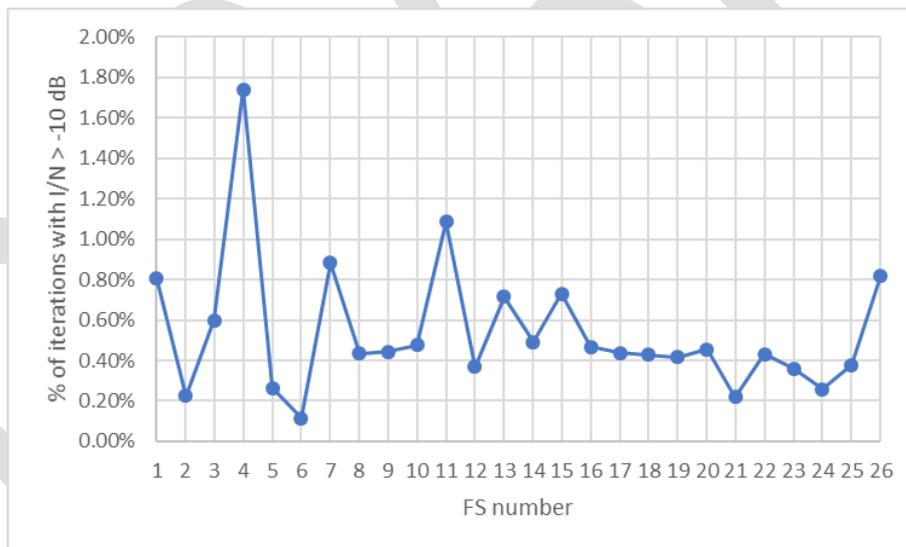
**Figure 36: Statistics of aggregate I/N > -10 dB for each of the 26 FS receivers in the Netherlands**
