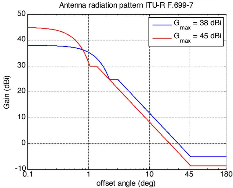
**Figure 5: Antenna radiation pattern of PP FS system for single-entry interference according to Recommendation ITU-R F.699-7 at the band centre frequency of 6.175 GHz**
