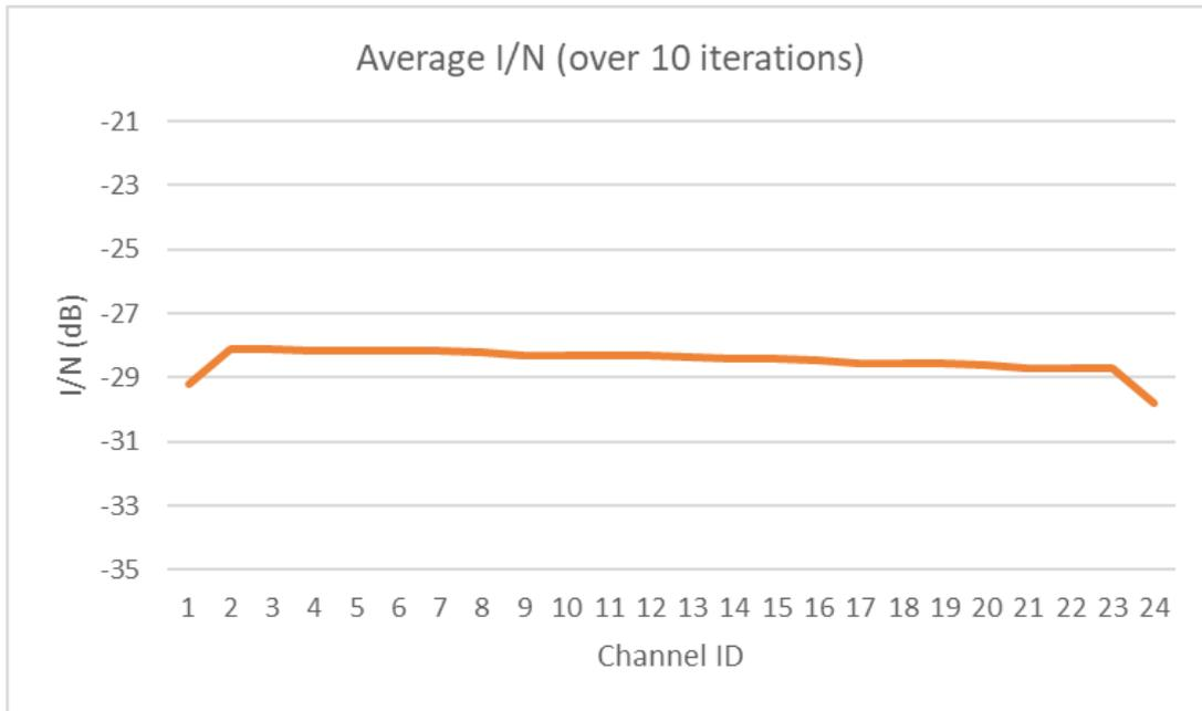
**Figure 62: IS-14 I/N per channel under mid active RLAN assumptions**
