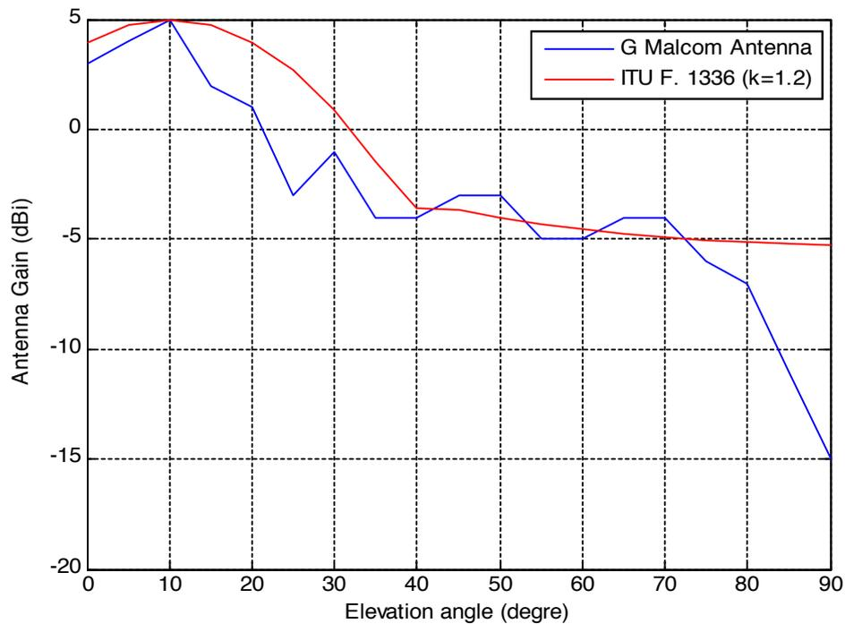
Figure 78: ITS OBU and RSU antenna pattern
