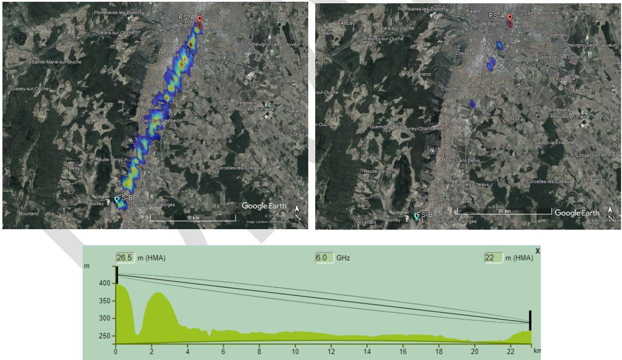
Figure 51: Fixed link 2 at Dijon. Top left: Outdoor RLAN impact on the fixed link, Top right: Indoor RLAN impact on the fixed link. Bottom: Fresnel zone and path profile
