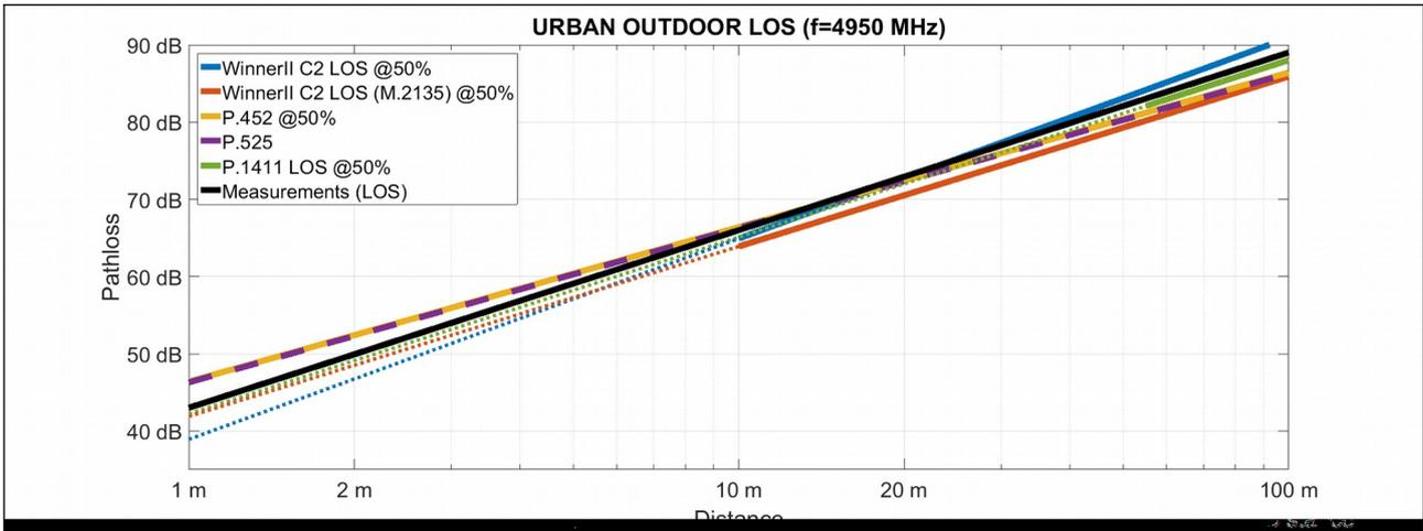
**Figure 116: Comparison of propagation models**
