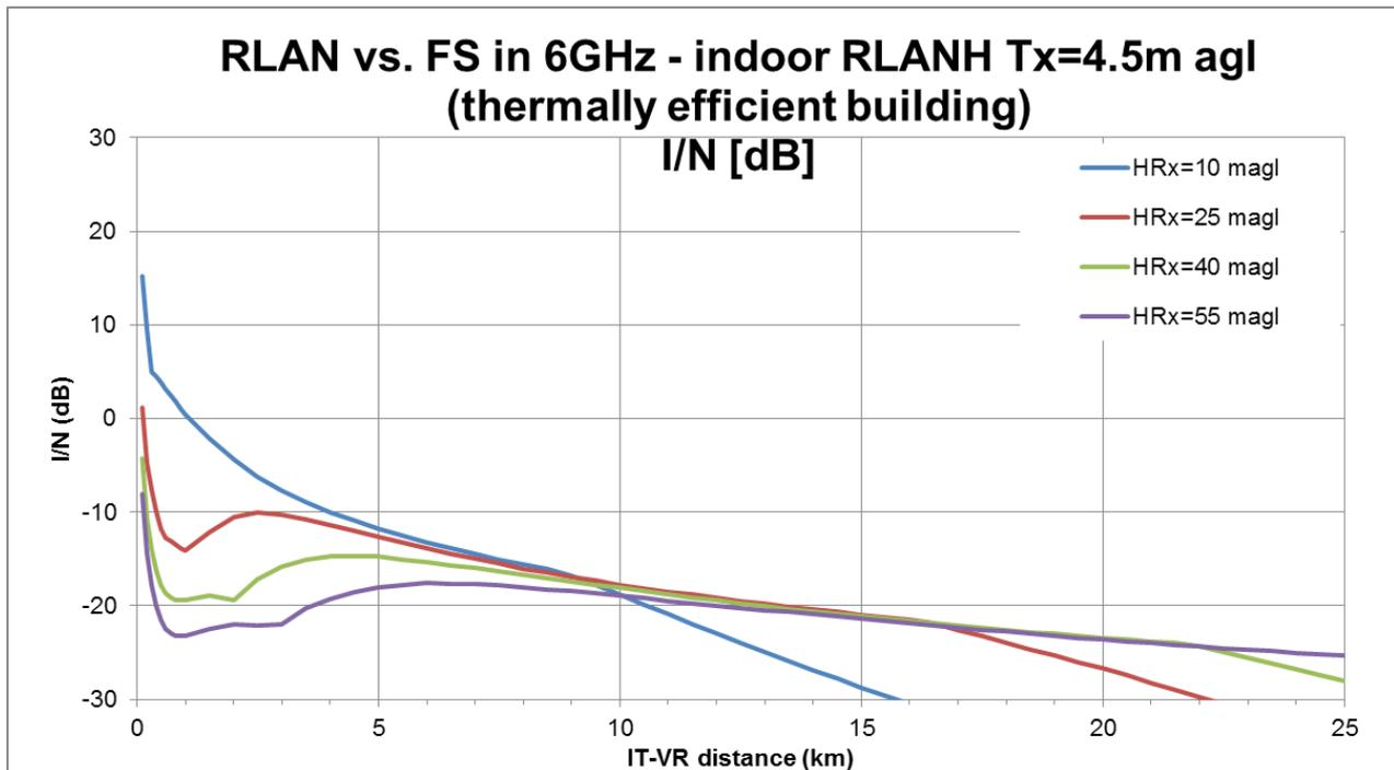
Figure 27: I/N at FS in dependence of RLAN distance in 0° azimuth direction of FS main beam (indoor RLAN @ 4.5 m, thermally efficient building type)
