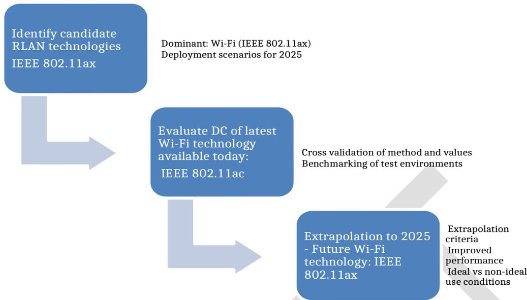
**Figure 123: Process applied to estimate the 6 GHz RLAN duty cycle**
