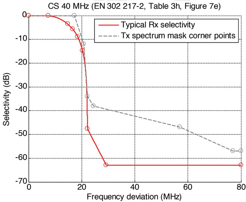
Figure 8: Typical receiver selectivity mask for FS systems with channel spacing 40 MHz
