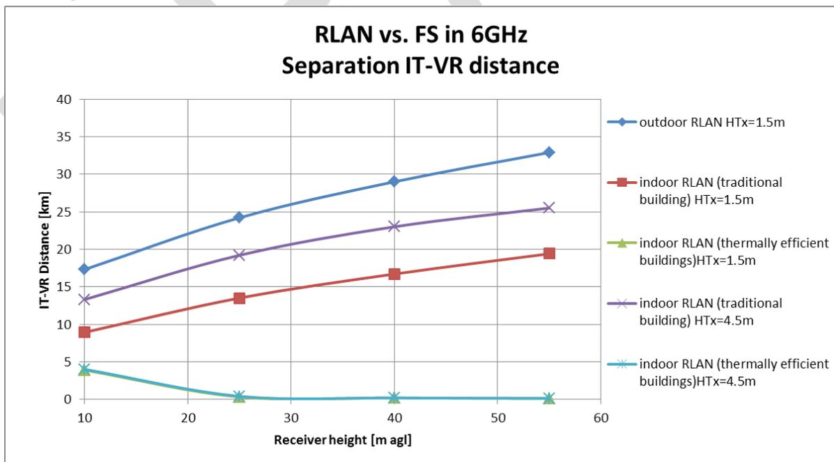
**Figure 30: Dependency of critical peak radii on the FS receiver height and RLAN environment for  $I/N = -10$  dB and maximum interference scenario**
