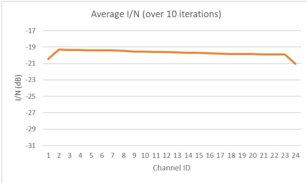
**Figure 60: IS-35E I/N per channel under mid active RLAN assumptions**
