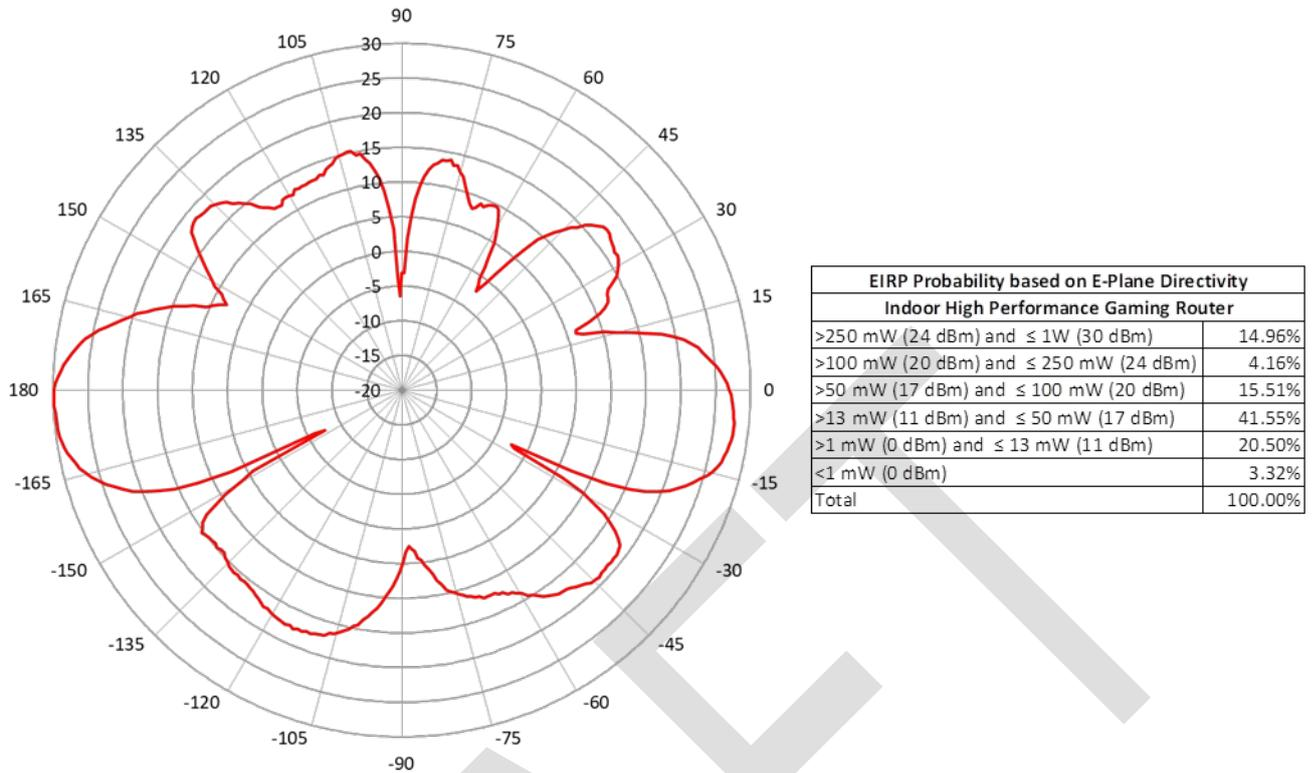
Figure 103: e.i.r.p. probability based on E-plane directivity for indoor high performance gaming router
