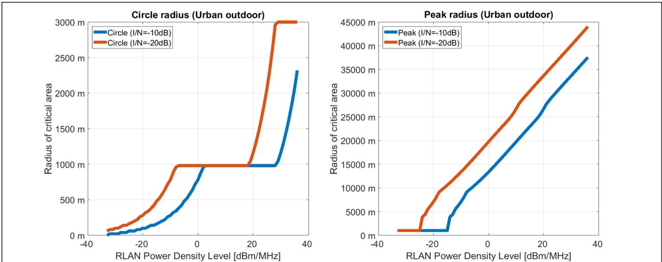
**Figure 29: Dependency of critical radii on the RLAN power density outdoors**
