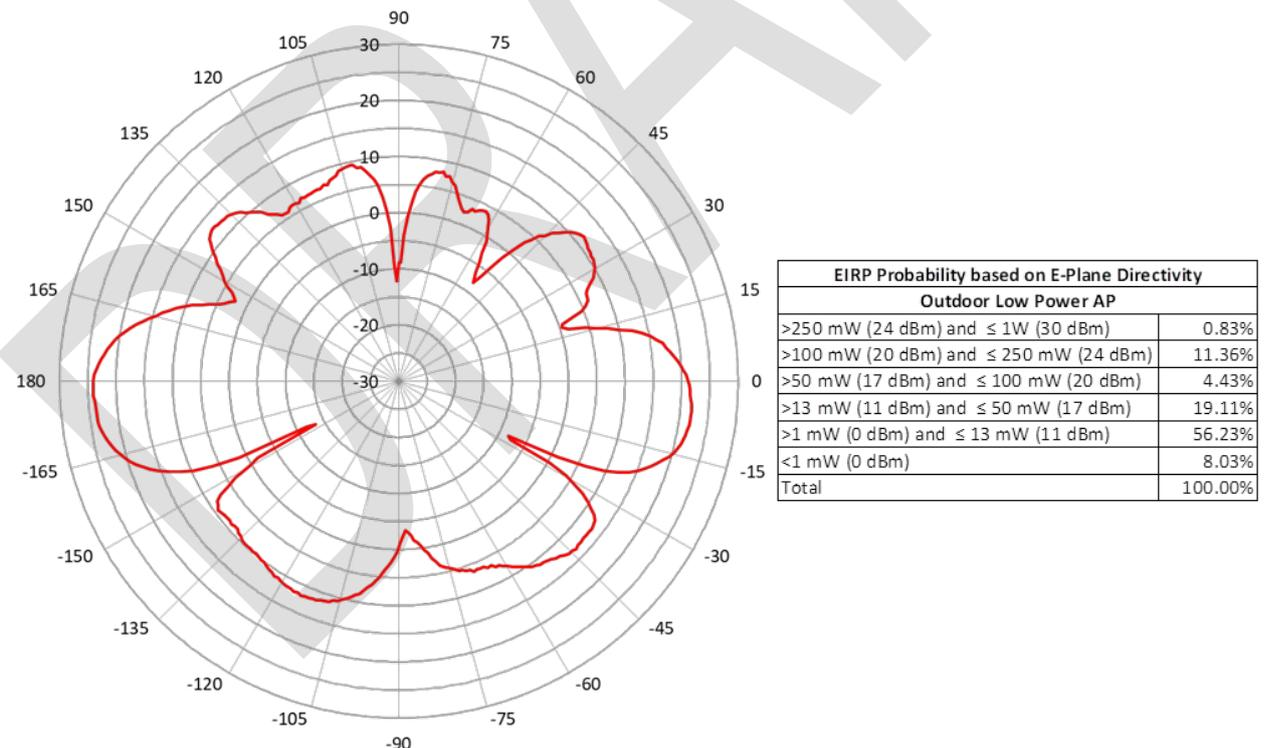
Figure 106: e.i.r.p. probability based on E-plane directivity for outdoor low power AP
