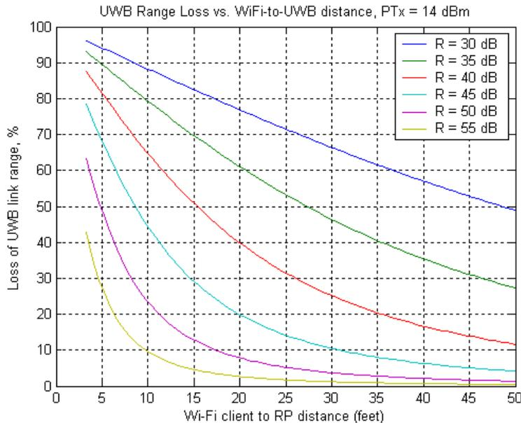
**Figure 93: UWB range loss versus separation distance**
