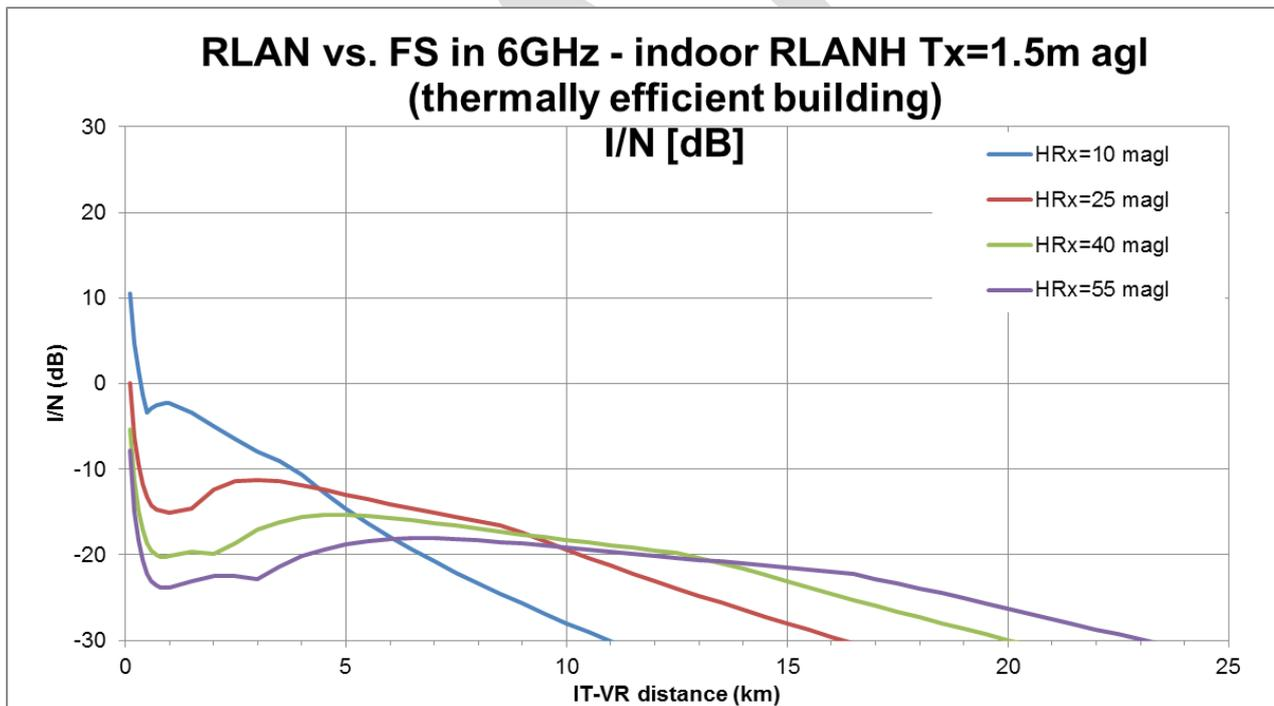
Figure 26: I/N at FS in dependence of RLAN distance in 0° azimuth direction of FS main beam (indoor RLAN @ 1.5 m, thermally efficient building type)
