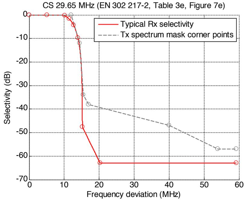
**Figure 10: Typical receiver selectivity mask for FS systems with channel spacing 29.65 MHz**
